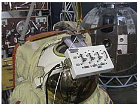
Image above: A control panel on the outside of the space suit will let the crew activate Suitsat-1 when it's deployed. Credit: NASA
