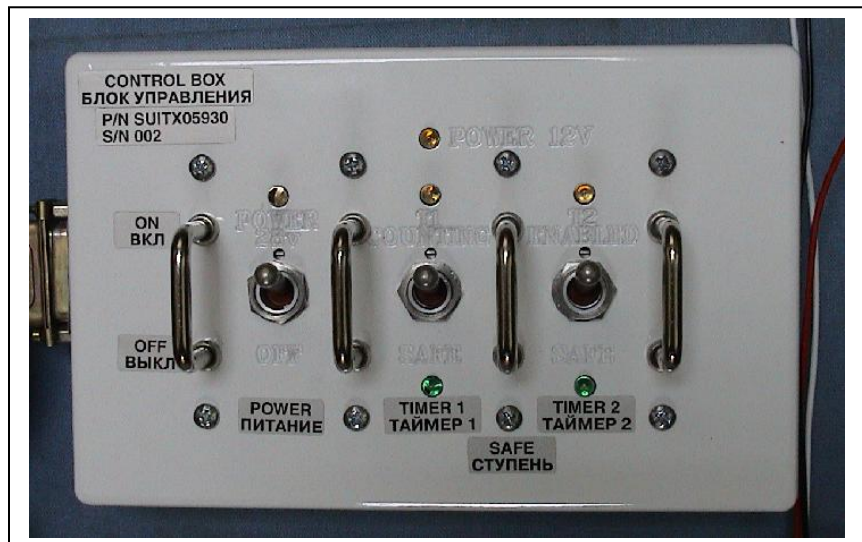
Figure 5 - SuitSat 1 Switch Box
