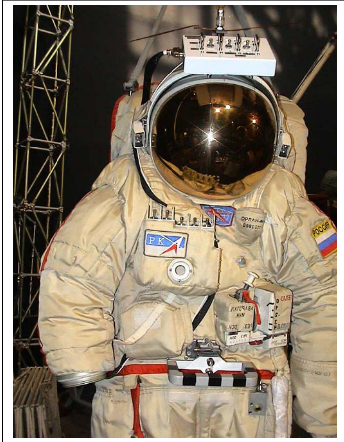
Figure 1 - SuitSat is a Russian Orlan spacesuit fitted with an antenna and activation switches on the helmet. The radio and batteries are inside the suit. (Photo courtesy RSC Energia)
