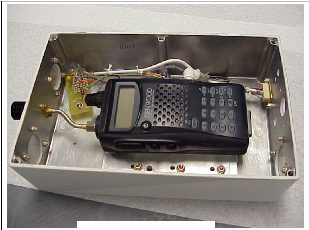
Figure 3 - SuitSat 1 Radio Box.
