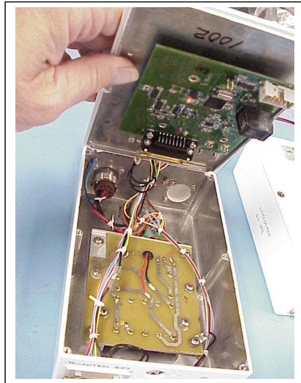
Figure 4 - SuitSat 1 Controller Box. The controller PCB is on the lid. The EMI filter and DC-DC converter are inside the box.
